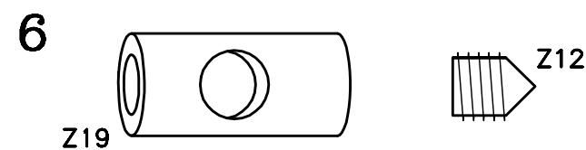
If the leg is loose after assembly, loosen the screw Z12 slightly, until the lower leg can be turned 1 time around clockwise. Then tighten the Z12 screw again.
