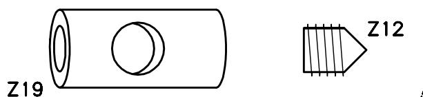
If the leg is loose after assembly, loosen the screw Z12 slightly, until the lower leg can be turned 1 time around clockwise. Then tighten the Z12 screw again.
